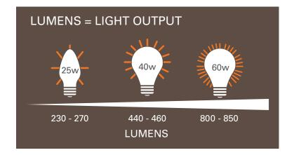
For non-directional bulbs, such as a globe or candelabra, the total lumen output is calculated in all directions. With a directional bulb, such as a spotlight, the light is emitted in many directions, some of the light (spill light) may not be useful but it is counted in the total lumen rating.
